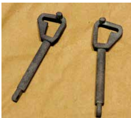
Door rods cast in aluminium alloy as an aftermarket, stronger version.
