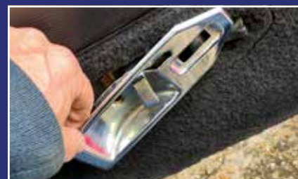
Then remove the escutcheon trim from the inner door handle.
